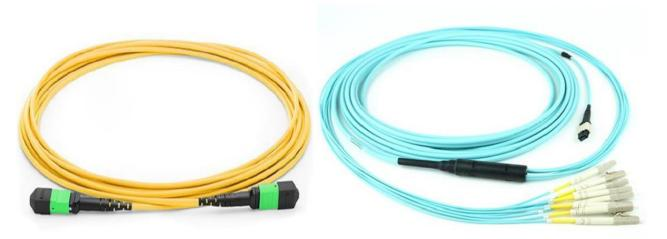
This patch cord consists of a free-form cable where fibers with a 250 $\mu$ m sheath are inserted into one or more tubes. This cable is protected by a halogen-free, low smoke sheath. In the case of a hybrid octopus, a spark gap allows the duplex fibers sheathed in 900  $\mu$ m, then over sheathed in 3mm to exit, to then mount an LC connector at each end of the fiber.
